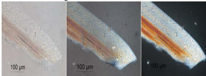
Figure 2: Polyester fibers damaged with a nail gun viewed under plane polarized light (left), 65° crossed polarizers (middle) and 90° crossed polarizers (right). Magnification x400.
