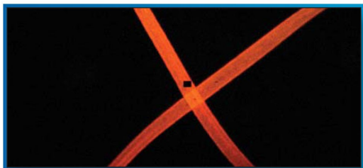
Fluorescence imaging of a nylon fiber with CRAIC's unique calibrated variable aperture.
