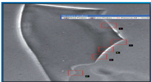
Glass fragment with multiple probes for fast and accurate quantification measurements.
