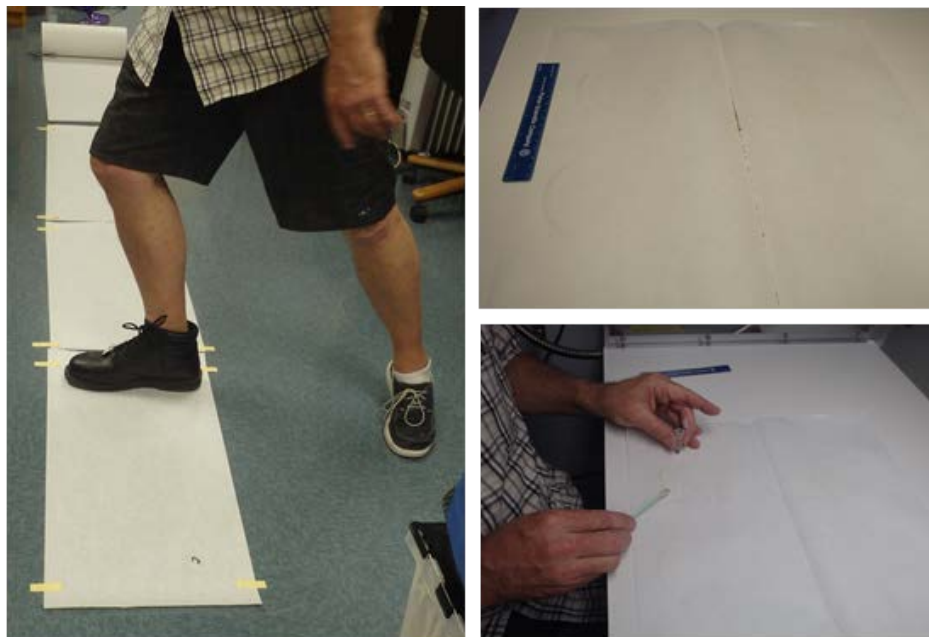
Figure 1: Removal of the most loosely held particles by walking on paper.
