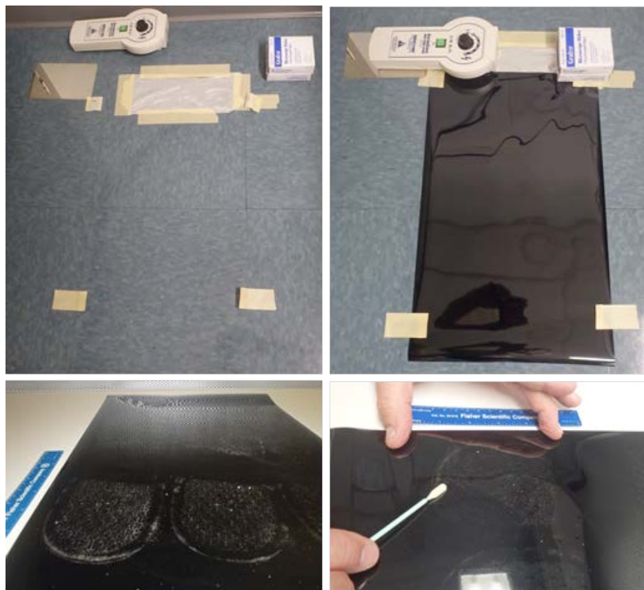
Figure 2: Removal of moderately held particles using an electrostatic lifter.
