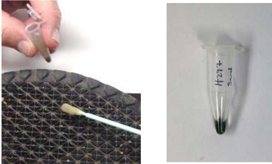
Figure 3: Removal of the most tightly held particles by direct swabbing of contact surfaces of the sole.
