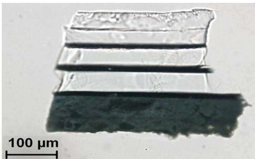
Figure 7: Manual cross section of a 9-layer paint chip (using both transmitted and reflected lighting) where two OEM factory repair topcoats are further covered by an aftermarket clearcoat refinsh. From the bottom of the chip, medium gray e-coat (OU2), dark gray primer surfacer
