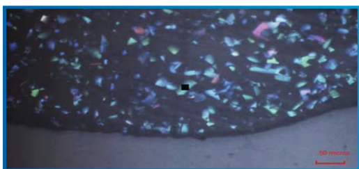
Chromaffair paint sample using 10x magnification in reflectance, microscale shown is 50 microns.
