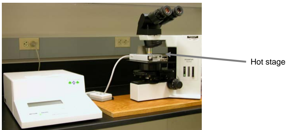
Figure 4: A photograph of the Mettler Hot Stage equipment and microscope used in Study 4.
