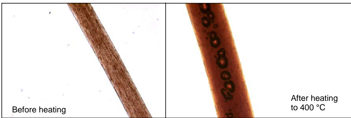
Figure 5: Two photomicrographs of a hair from Study 1. This hair was exposed to a temperature of 400 °C. Color change, expansion, and bubbling are evident. Both photos were originally taken at 400x magnification.
