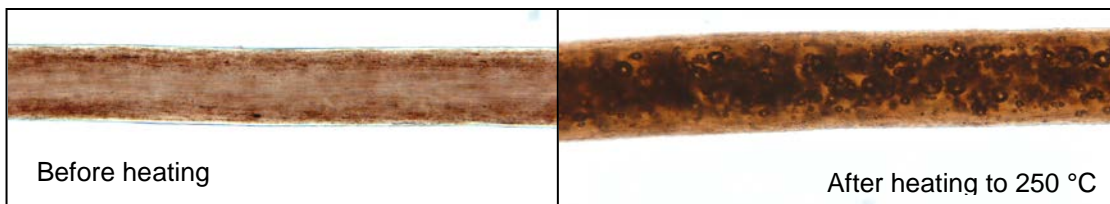
Figure 7: Two photomicrographs of a hair from Study 4. This hair was exposed to a temperature of 250 °C. Color change, expansion, and bubbling are evident. Both photos were originally taken at 200x magnification.
