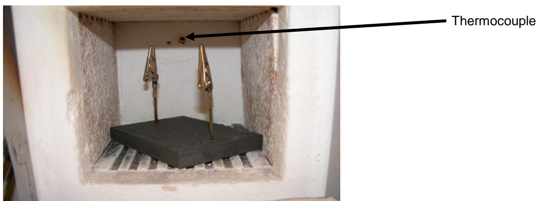
Figure 3: A photograph of the apparatus inside the oven for Study 3. The diagonal orientation of the metal block and the test hair with respect to the oven walls and thermocouple is shown. Study 2 was set up similarly, except for the orientation of the metal block.
